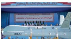
to the operational specifications required by the Air Force of the Army, and it carries 4 bombs of the Qaem class, in addition to two smart missiles, and it was also equipped with the X-Band jamming system.
